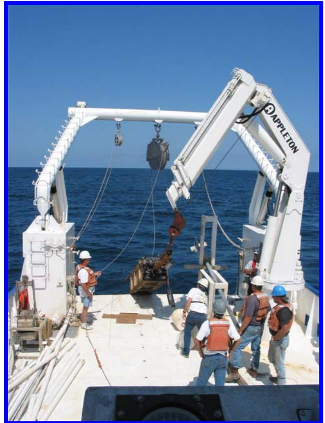
**Figures 5 and 6.** Prototype geophysical array with ROV replaceable DATS (left). Geophysical array readied for deployment (right).
