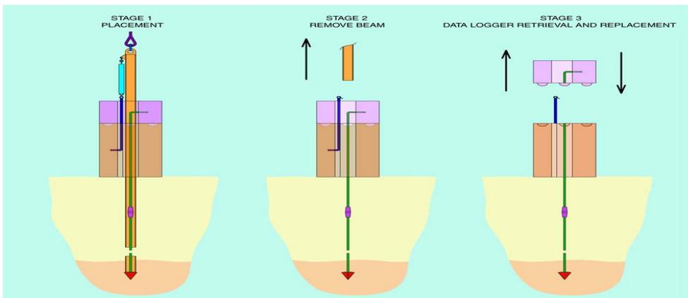
**Figure 7.** Conceptual drawing of Sea Floor Probe installation.
