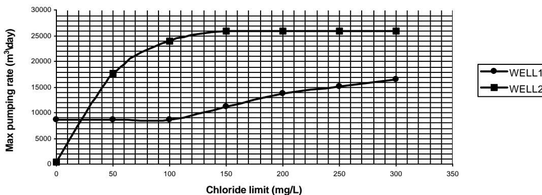
Figure 5: Trade-off curves between maximum pumping rate and chloride concentration limit
