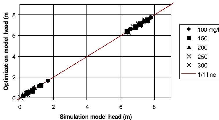
Figure 3: Correlation between simulation model results and optimization model results for hydraulic heads.
