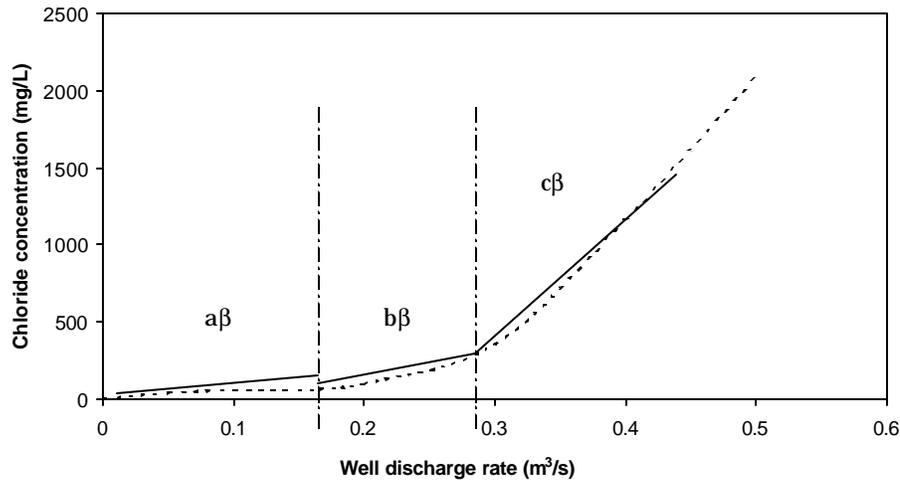
Figure 2: Chloride concentration versus discharge and estimation of chloride concentration influence coefficients.
