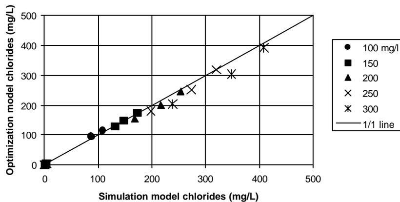
Figure 4: Correlation between simulation model results and optimization model results for chloride concentrations.
